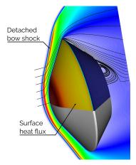
For this application, a generic spacecraft geometry is simulated with the Direct Simulation Monte Carlo (DSMC) module of PICLas. The incoming free-stream conditions are derived at the point of peak heating from an exemplary aerocapture trajectory. The hypersonic flow at a Mach number of 20 results in high-enthalpy conditions with a detached bow shock and a rarefied region behind the capsule. The figure shows the translational temperature in the symmetry plane and flow streamlines.
