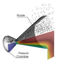
Large density gradients within the cold gas thruster ranging from continuum flow in the pressure chamber up to free molecular flow in the far wake of the nozzle pose a great challenge for a single numerical method. For this purpose, the Direct Simulation Monte Carlo (DSMC) module and the particle-based ellipsoidal statistical Bhatnagar-Gross-Krook (ESBGK) method of PICLas were coupled to exploit the advantages of both methods. While the DSMC method offers accurate
